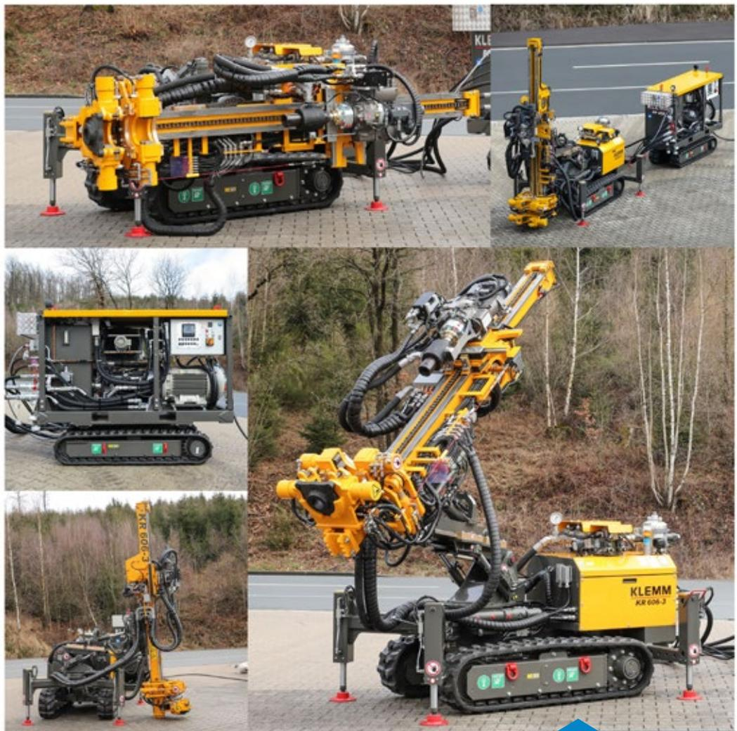
DEMONSTRATION OF POSSIBLE DRILLING POSITIONS © KLEMM BOHRTECHNIK GMBH
